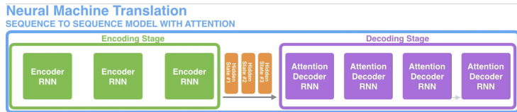
Figure 6: Attention model encodes information into sequence of vectors not in a single context vector, and chooses a subset of these vectors adaptively while decoding the translation.
